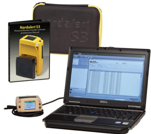
Front to Back: Nardalert S3 hooked up to a personal laptop, Instruction Manual and NBM-TS Software, and Soft Carrying Case
