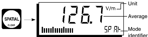
Figure 4-31 “Spatial Averaging” mode for determining the average field strength within a spatially extended area
