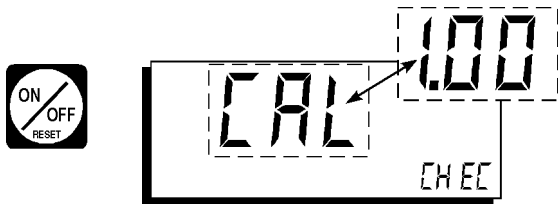
Figure 4-4 The self-test runs immediately after switch-on
