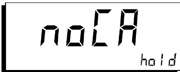
Figure 4-20 No calibration data for the current probe was found.
