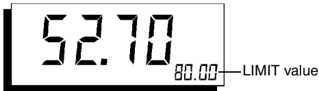
Figure 4-8 Display (using weighted frequency response probe as example) The display shows the power density expressed as a percentage of the limit value specified in the relevant standard.
