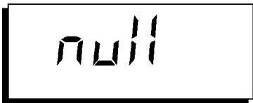
Figure 4-17 Display during automatic zeroing
