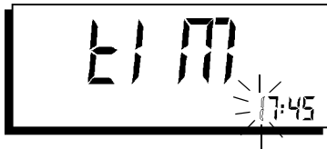
Figure 4-34 Entering the time of day; the digit being edited flashes
