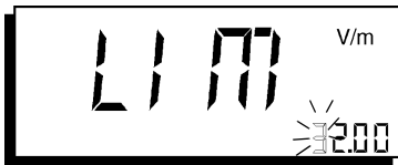
Figure 4-11 LIM indicator. The digit which can be altered flashes in the display.
