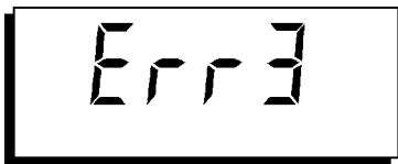
Figure 4-18 An error was detected during the self-test.
